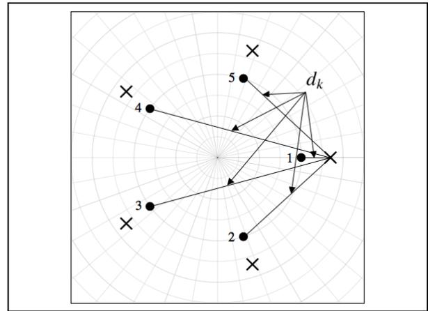
Figure 4. Distance  $d_k$  from worker to each source in system.
