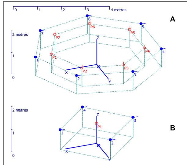
Figure 7. A) Model of the station for simulation based on assumptions from section 3.1. for  $W=7$ ;  $R=2m$ ;  $d_W=0.7m$  and B) its substitute model. Calculated substitute distance equals  $1,6m$ .
