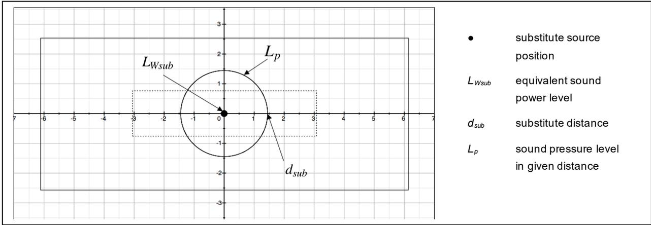
Figure 2. Proposed substitute model of the station with substitute source and substitute distance.
