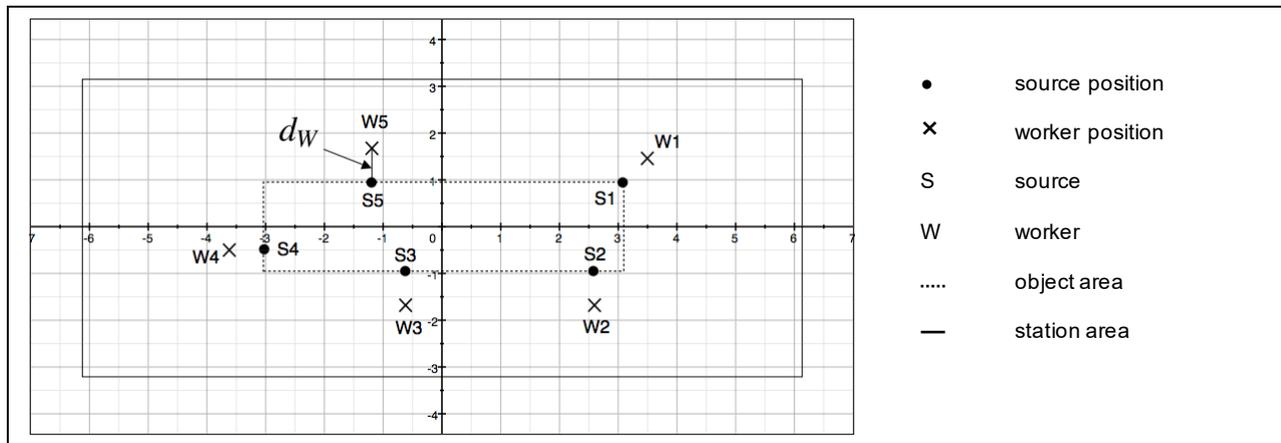
Figure 1. Possible setup of sources (S) and workers (W) on the station for a random moment of production cycle, where dots mark the position of sources and crosses mark the position of workers. Grid in metres.
