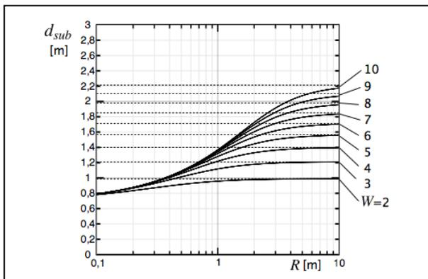
Figure 6. Substitute distance varies depending on the number of workers for constant source-worker distance  $d_W=0.7m$ . Dotted line shows upper limit value of  $d_{sub}$ , see equation (3).
