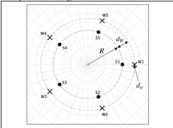
Figure 3. Detailed model of the station, where ● – (S)ources, × – (W)orkers,  $R$  – radius of sources setup,  $d_o$  – radius of workers setup,  $d_w$  – source-worker distance.
