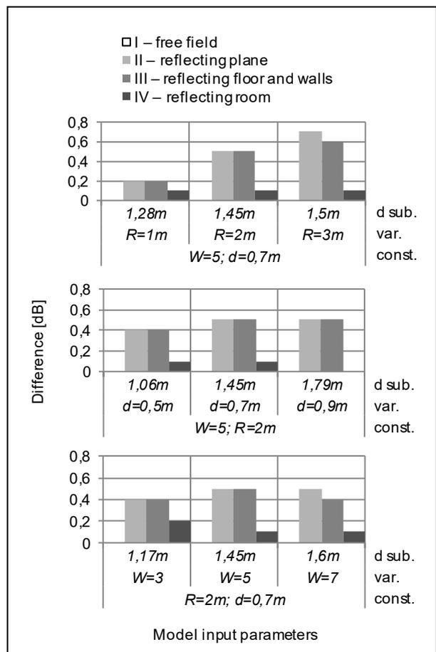
Figure 8. Difference between average sound level at operator's position calculated using substitute model and assumed model of the station: variable  $R$ , variable  $d$ , variable  $W$ . I-IV – variants of adaptation,  $W$  – number of workers,  $R$  – radius of the object,  $d=d_W$  – source-worker distance.
