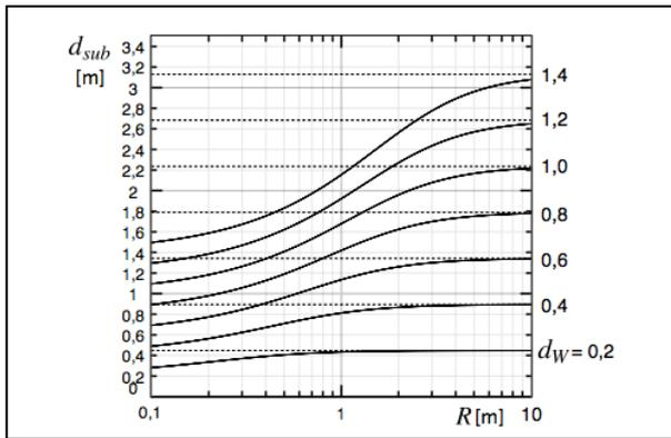
Figure 5. Substitute distance varies depending on average distance between operator's position and his source for constant number of workers  $W=5$ . Dotted line shows upper limit value of  $d_{sub}$ , see equation (3).
